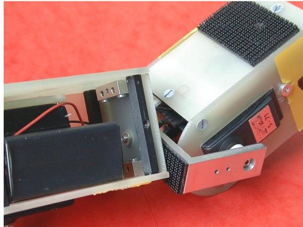
**Figure 2.7.:** Two modules connected in 45 ° orientation
