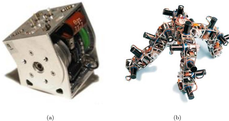
**Figure 1.3.:** Polybot G3 prototype (a) and G2 in spider configuration (b)
