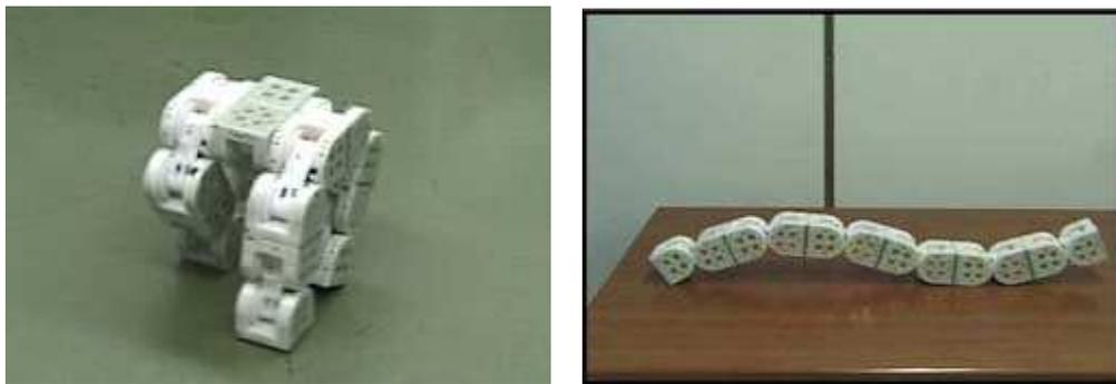
Figure 2: M-TRAN II configured as quadruped and caterpillar.
