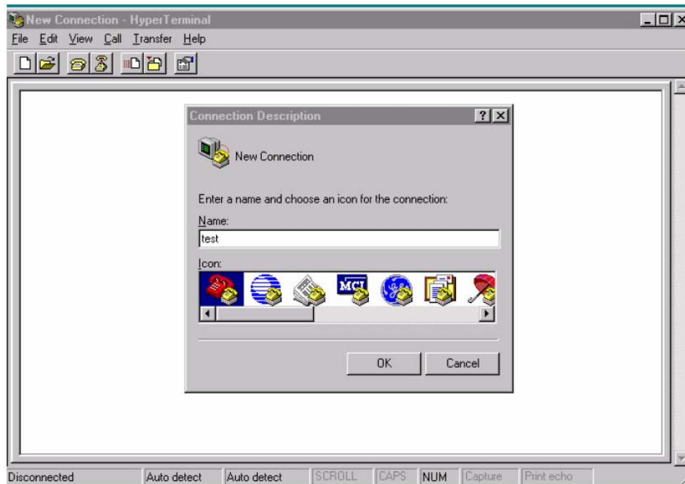
Figure 3: Create new connection in Hyper Terminal
