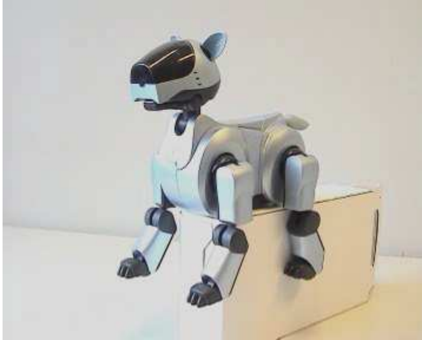
Figure 3.2: Experiment setup in reality This photos shows the AIBO laid on a white cardboard box. Such a setup allows its legs to move freely without touching the ground or other objects.
