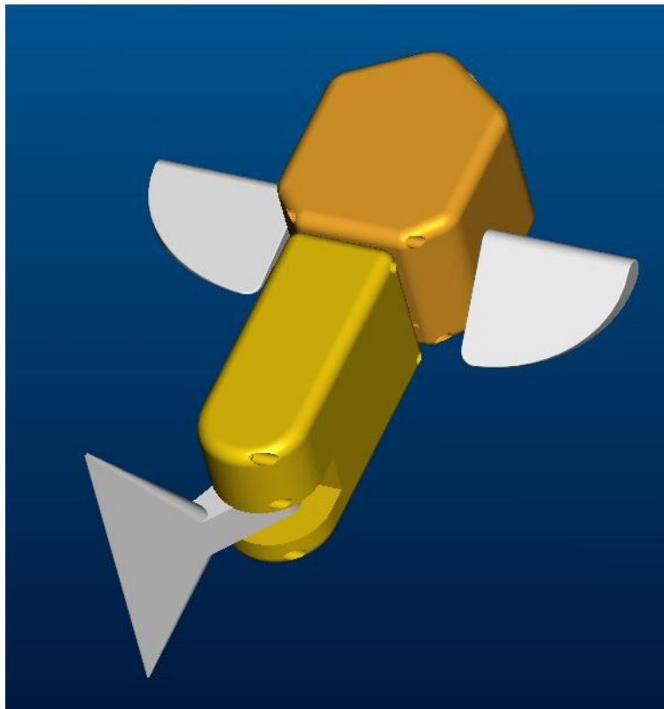
Figure 3.3: Fish robot designed for ostraciiform or labriiform swimming mode
