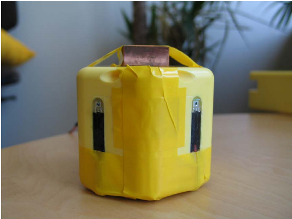
Figure 4. Head/flipper module with photo sensors mounted on the face. A copper weight was used to keep the module from floating during tests.
