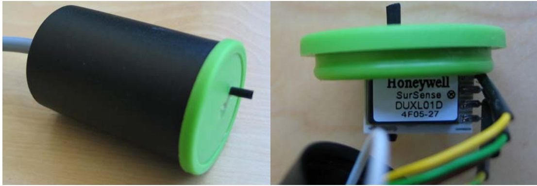
Figure 5. A plastic container in which the pressure sensor was tested is shown on the left. An image of how the pressure sensor was mounted to the lid is shown on the right.
