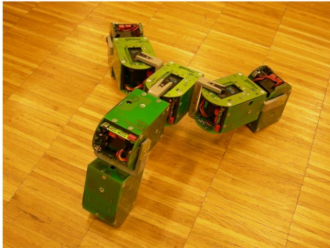
**Figure 1.4:** Example of a YaMoR structure
