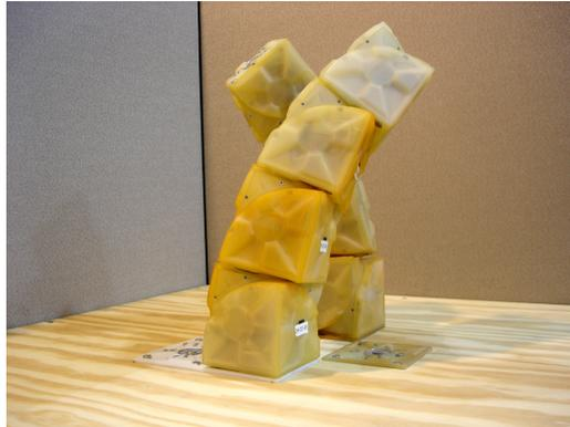
**Figure 1.2:** Example of a self-replicating robot: Molecube (Zykov *et al.*, 2005).
