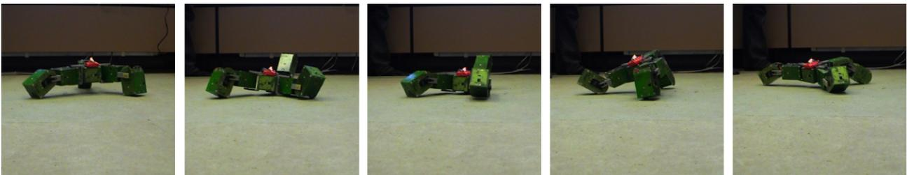
**Figure 4.8:** Snapshot of the evolved gait for the tripod robot.
