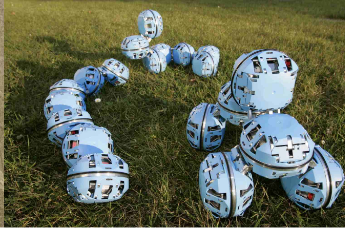
Figure 3.7: Several Atron configurations, including a car-like one. [10]
