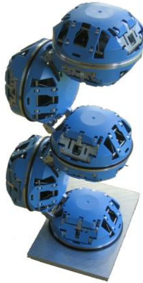
Figure 3.1: Lattice architected robot example: an assembling of Atron modules [1].
