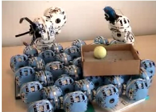
(a) the ATRON modules : a Lattice architecture
